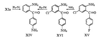
stance (XIV) was then identified with an authentic sample which was prepared by causing 2-amino-5chloro-4'-fluorobenzophenone (XV) to react with ammonia under pressure, and subsequent dehalogenation of the product XVI with hydrogen in the presence of a palladium catalyst.
